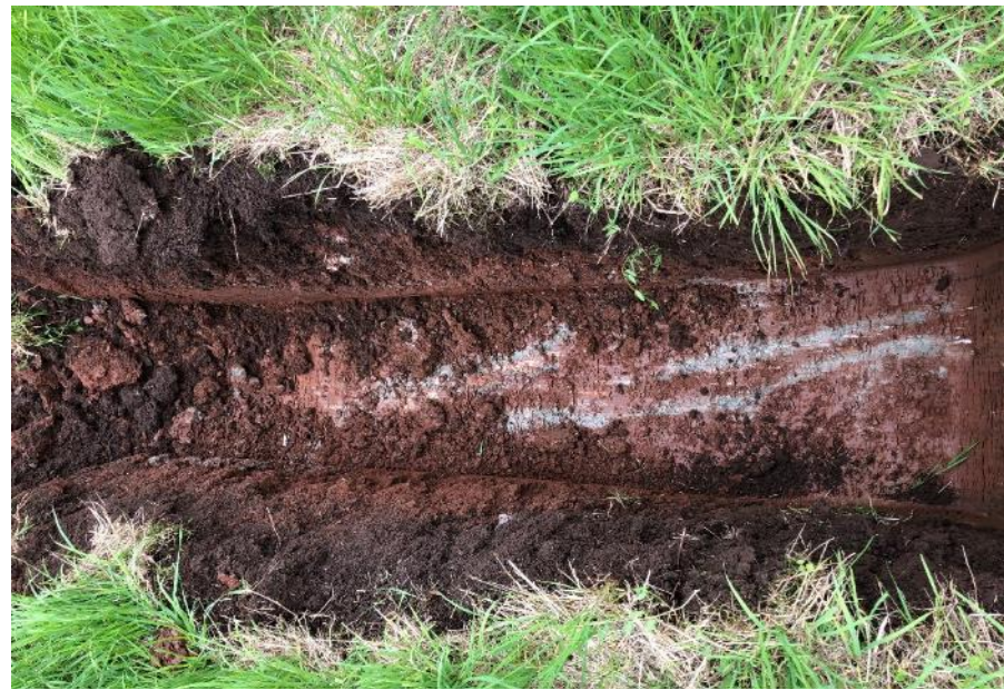
Photograph 4 – Displaying the in-situ shallow Mercia Mudstone Group, taken from TP04.
