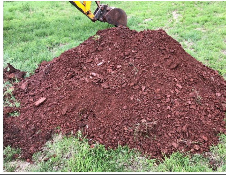
Photograph 2 – Displaying the underlying Mercia Mudstone Group excavated from TP01.
