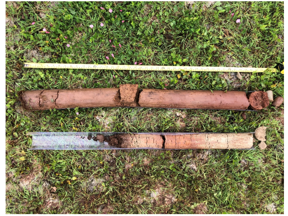
Photograph 3 – Displaying the underlying Mercia Mudstone Group strata from WS03, located in the historic pond area.
