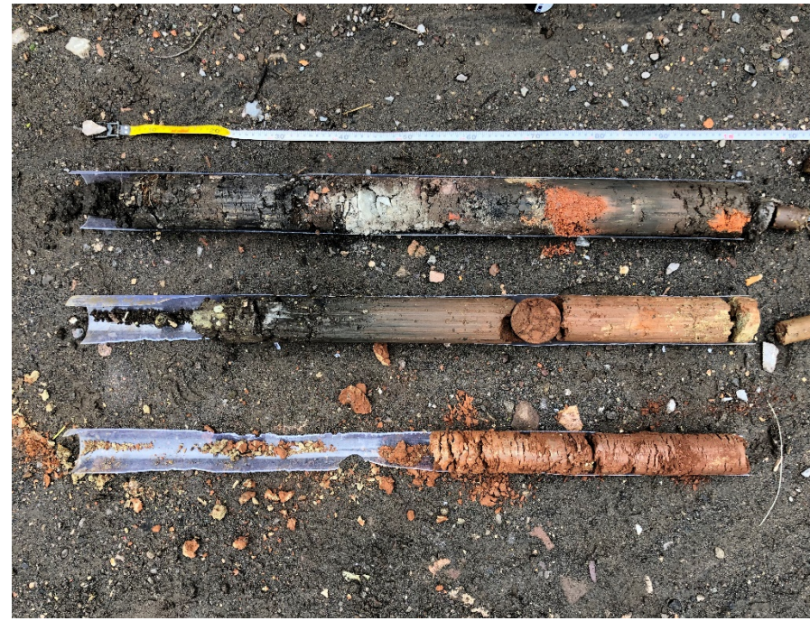
Photograph 2 – Displaying the underlying Made Ground (0.0m to 1.5m) and Mercia Mudstone Group (1.5m to 2.8m) at WS01.
