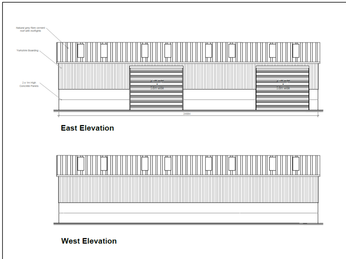
Figure 5: Proposed machinery store east & west elevations
