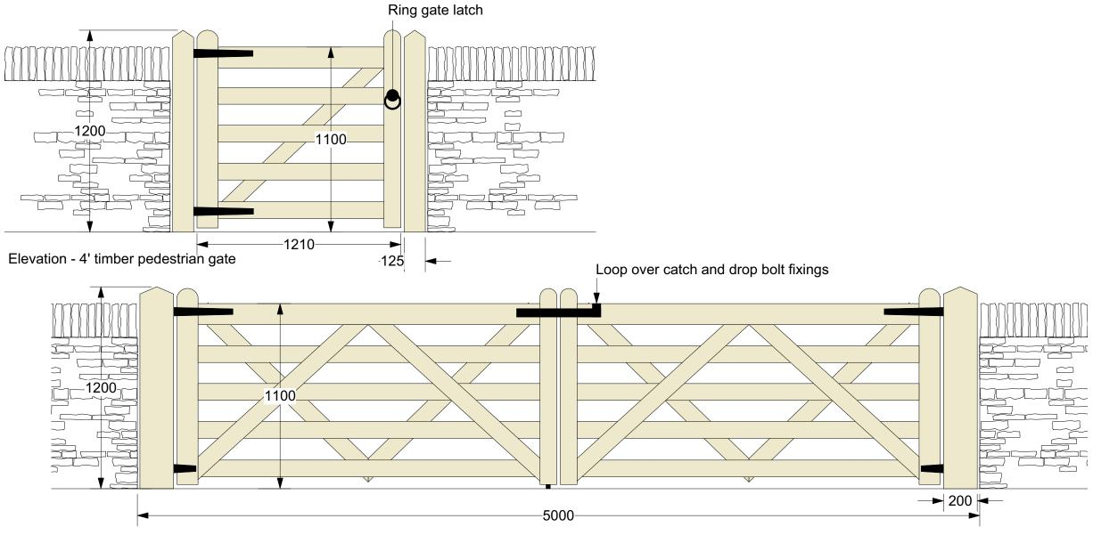
Elevation - Double timber driveway gate
