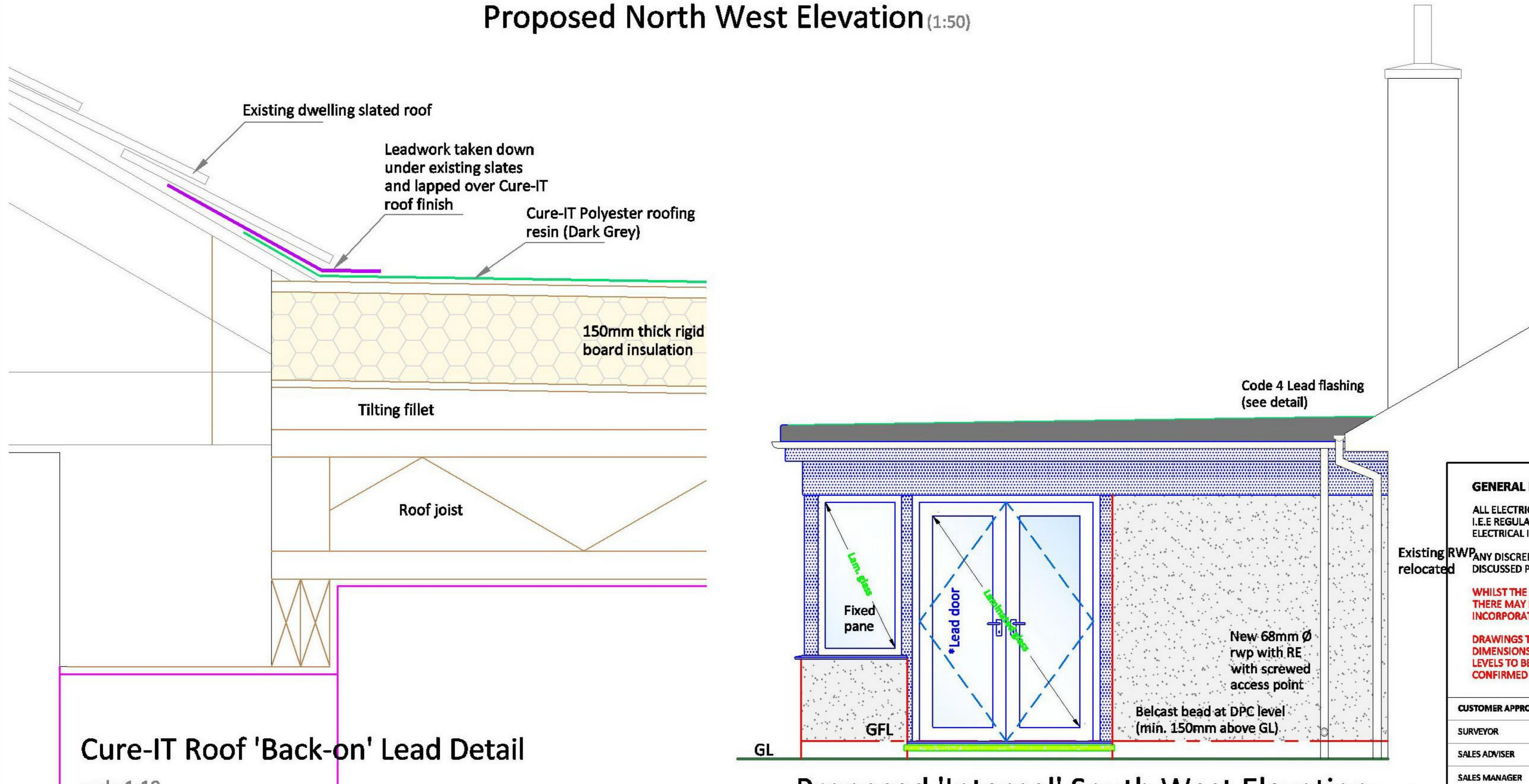
Cure-IT Roof 'Back-on' Lead Detail
