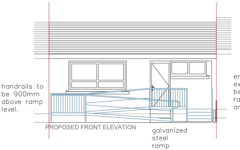
ensure handrails extend 300mm beyond end of ramp and steps and are rounded.
