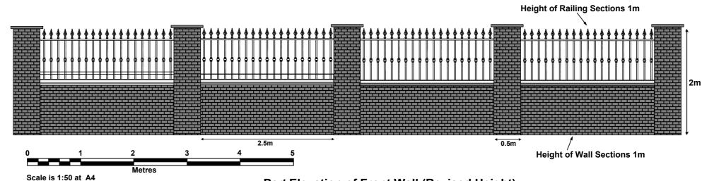
Part Elevation of Front Wall (Revised Height)
