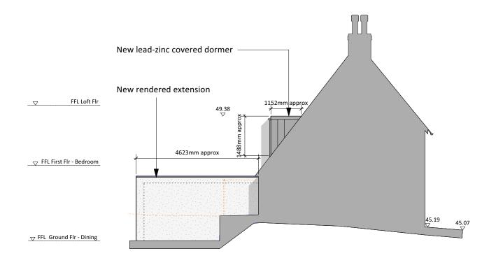
Proposed SE Side Elevation Scale: 1:100
