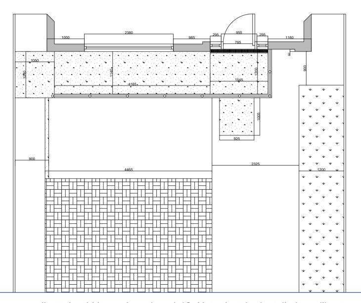
Ramp gradient should be no less than 1:12. Note that the installation will not be accepted if this gradient is not achieved and that remedial works will be at the contractor's expense.
