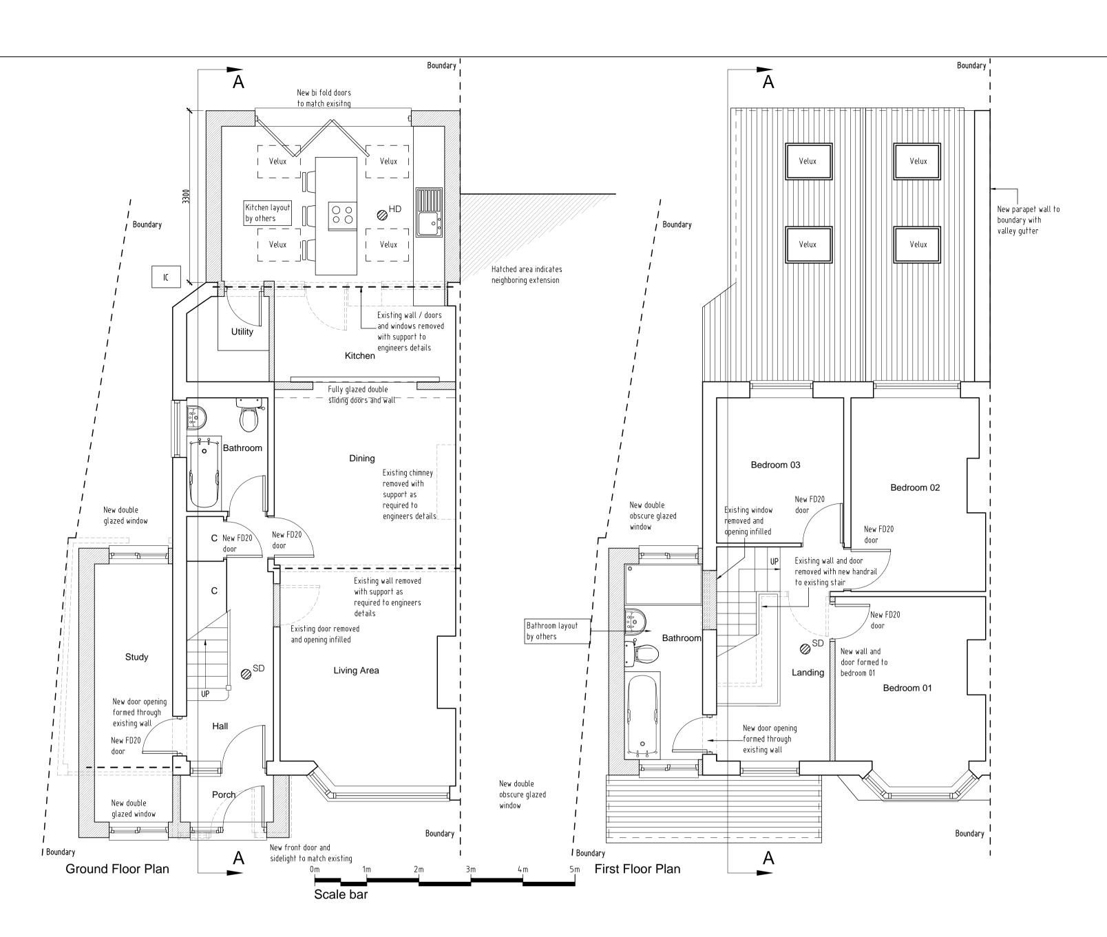
For proposed elevations see drawing 2020-119 - 004. Contractor to assume design responsibility under CDM2015. Note, all structural information noted should be checked against detailed structural engineers information / calculation sheets. Bedroom 03 Bedroom 01 Landing
