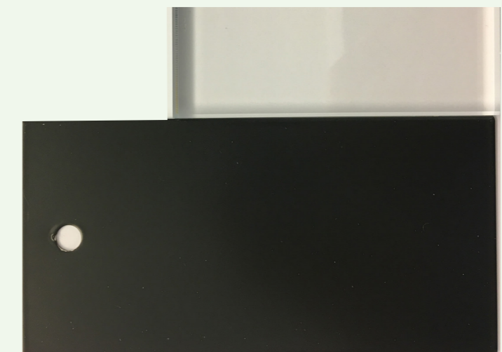
PROPOSED ANTHRACITE PPC FINISH TO CHAMBER STREET MANUFACTURER : TIGER - DRYLAC POWER COATINGS PRODUCT : 029/73570 MT/GL - RAL 7016
