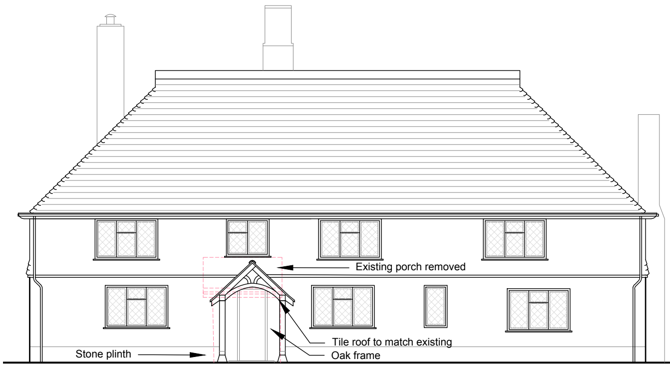
South West Elevation
