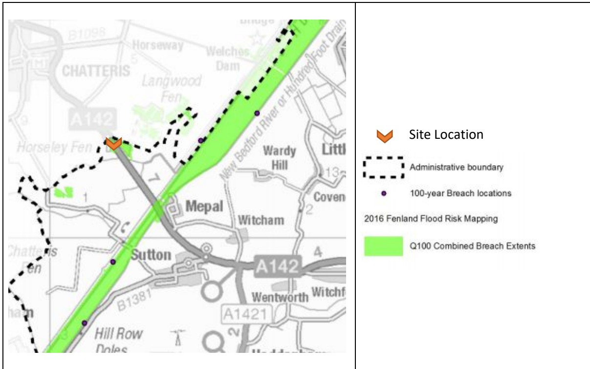
Figure 8. Map of East Cambridgeshire SFRA Flood Defence Maximum Breach Extent for a 1 in 100-year Event
