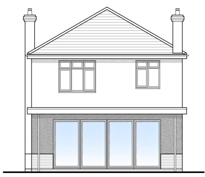
REAR ELEVATION AS PROPOSED | Scale 1:100 Painted brick and render to match existing dwelling
