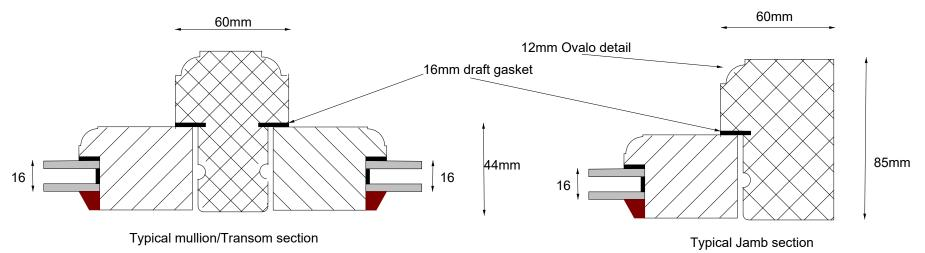
Generally 4.8.4 A rated edge units Argon filled soft coat warm edge spacer bar either silver or black to fit between glazing bars as individual units.
