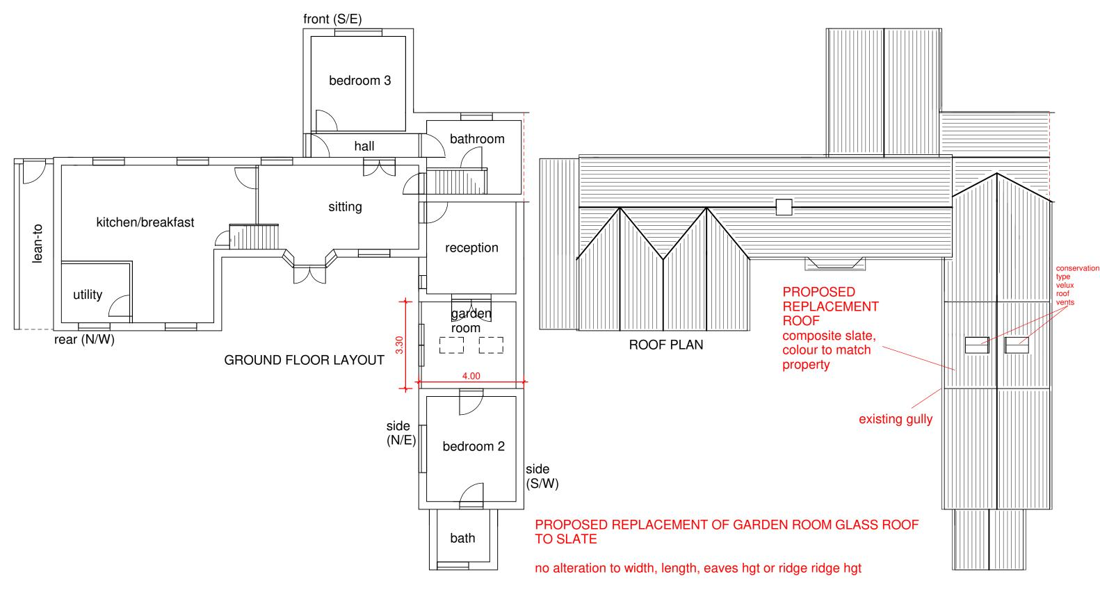
new roof to be composite slate, slate colour to match property, 2x conservation type velux roof vents, rainwater system black, drainage to existing gully
