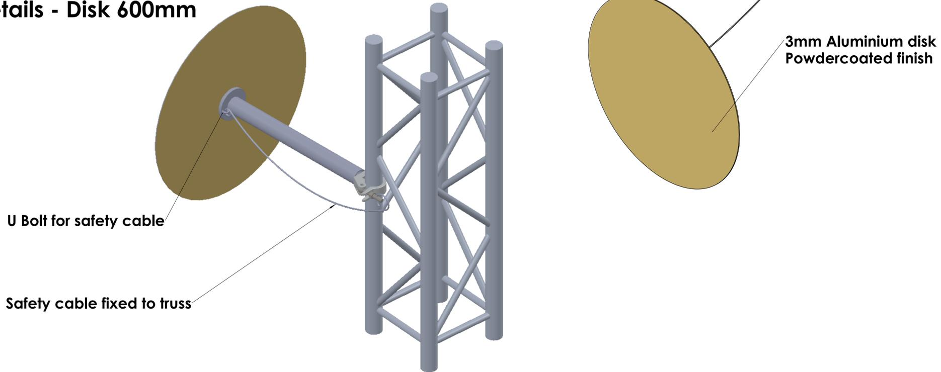
10mm Aluminium plate weld to disk with M12 bolt for arm
