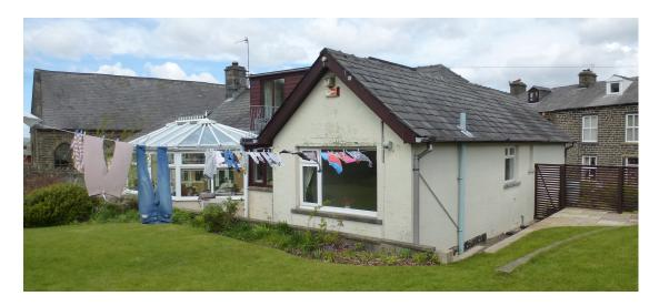
Note the existing ridge height running parallel with the road is raised higher than the ridge height over the existing ground floor bedroom accommodation. Also see Existing Southeast Elevation on drawing number 21-08-05.
