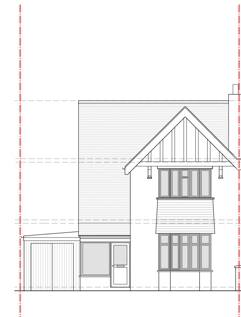
FRONT ELEVATION AS EXISTING
