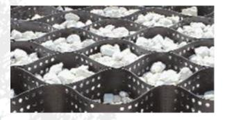
CellWeb is a three-dimensional cellular confinement system manufactured from high-density polyethylene (HDPE) strips that are ultrasonically welded together to create a strong, lightweight expandable panel.
