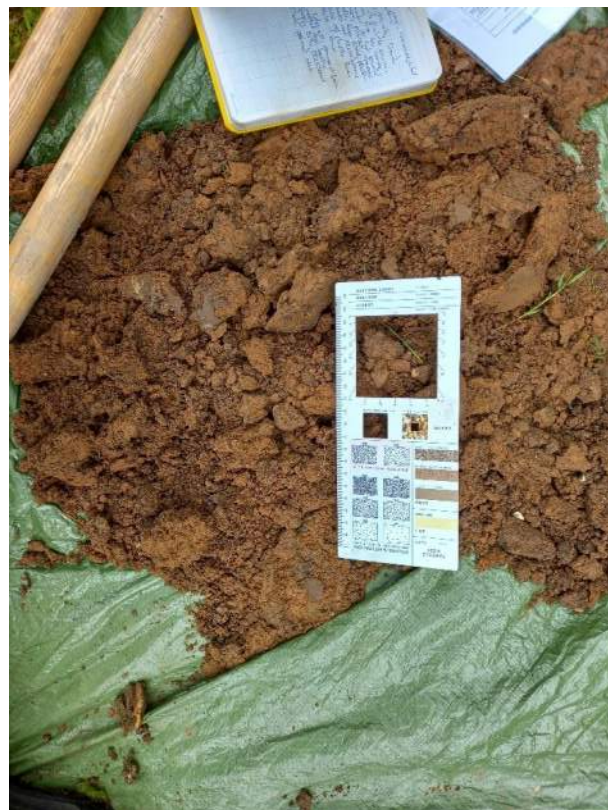
Photograph 16 – HP4 0.45 – 70m (NATURAL GROUND)
