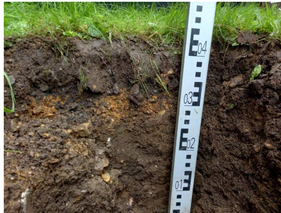
Photograph 14 – HP4 0.45m base of made ground. Made ground strata boundaries.
