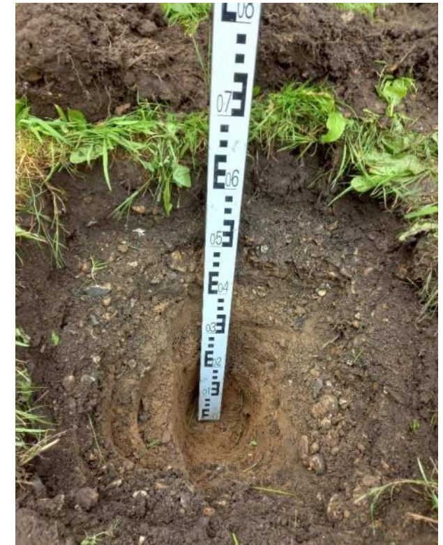
Photograph 3 – HP1 0.30 – 0.64m (NATURAL GROUND)
