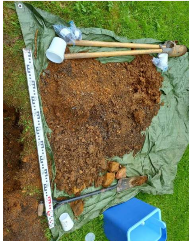
Photograph 7 – HP2 0.34 – 0.60m (NATURAL GROUND)
