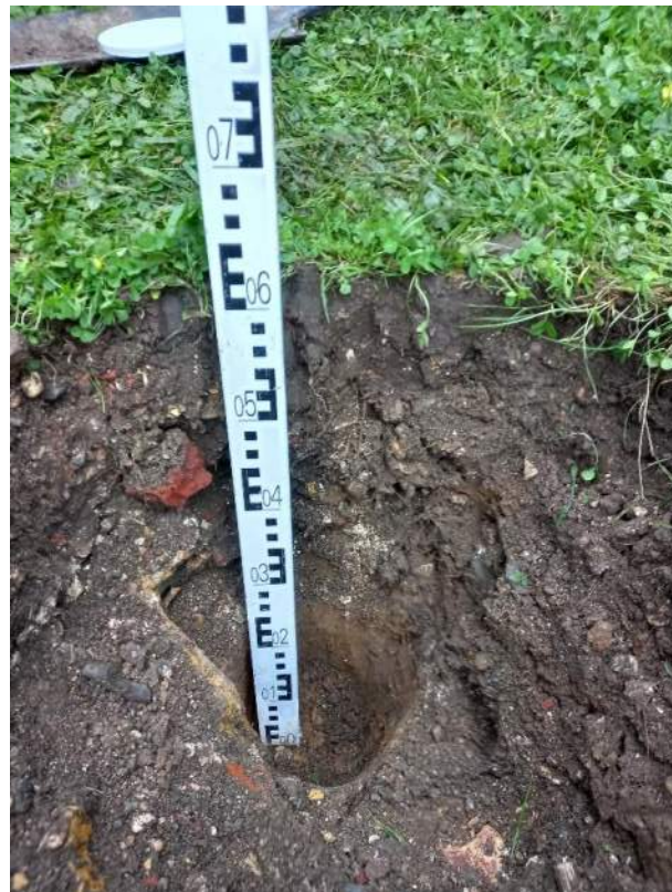
Photograph 10 – HP2 0.63m base. Made ground – natural ground boundary at 0.39m.
