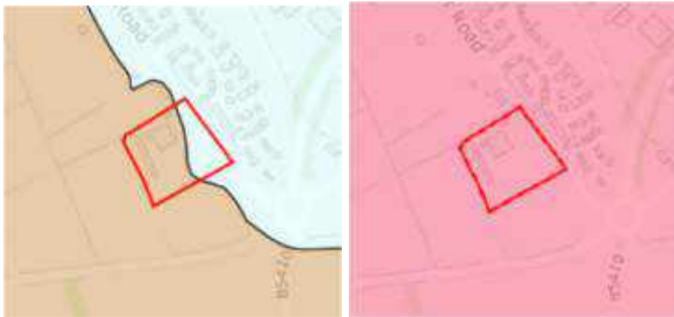
Figure 2; Extracts of the BGS 1:10,000 superficial and solid geological maps. Brown = Peat, Blue = Glacial Till and Pink = Kirkham Mudstone Member
