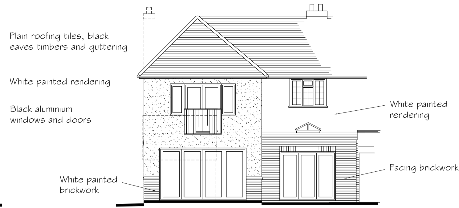
REAR (East) ELEVATION as proposed
