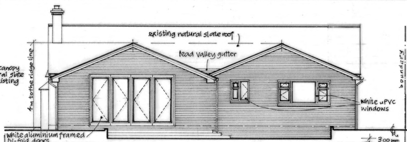
SOUTH WEST ELEVATION
