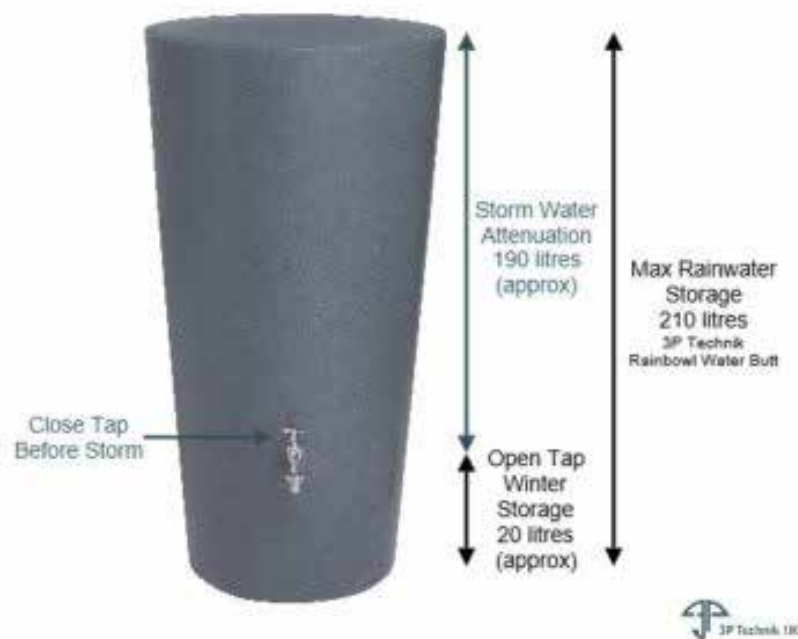
Fig 4 - Type of Household Water Butt Proposed
