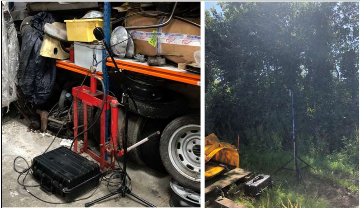
Figure 3. Sound Level Meter Monitoring Locations (Left-01dB SIP95/Right 01dB Black Solo)
