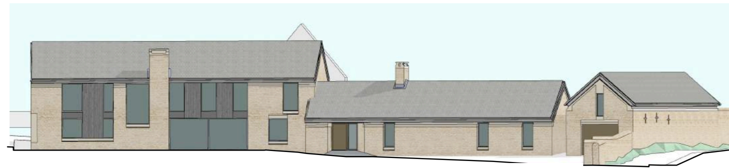
Proposed north elevation, left to right: new barn , rehabilitated stable, reconstructed cowshed
