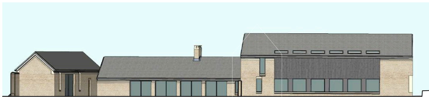
South elevation (with boundary wall and hedging not shown). Dashed line shows silhouette of listed barn
