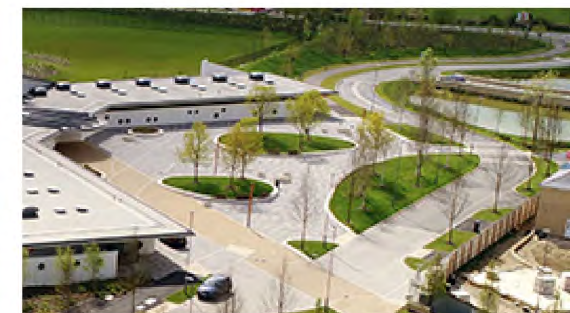
Example use of shaped grassed areas and tree planting to soften hard landscaped plaza area
