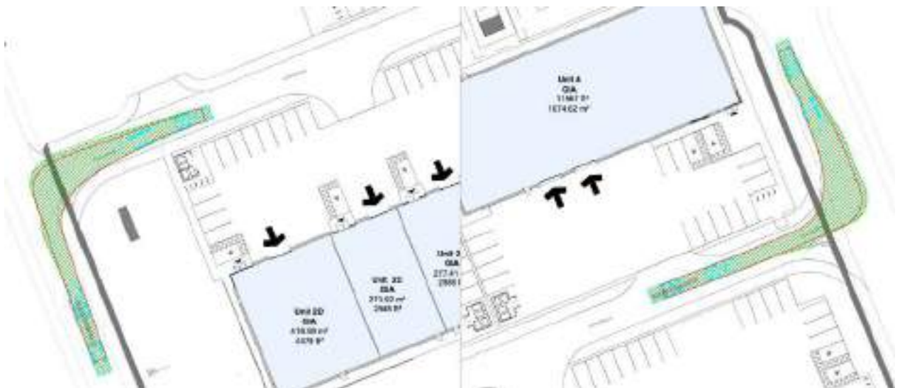
Figure 4.5: Swept Path Analysis – 16.5m Articulated HGV
