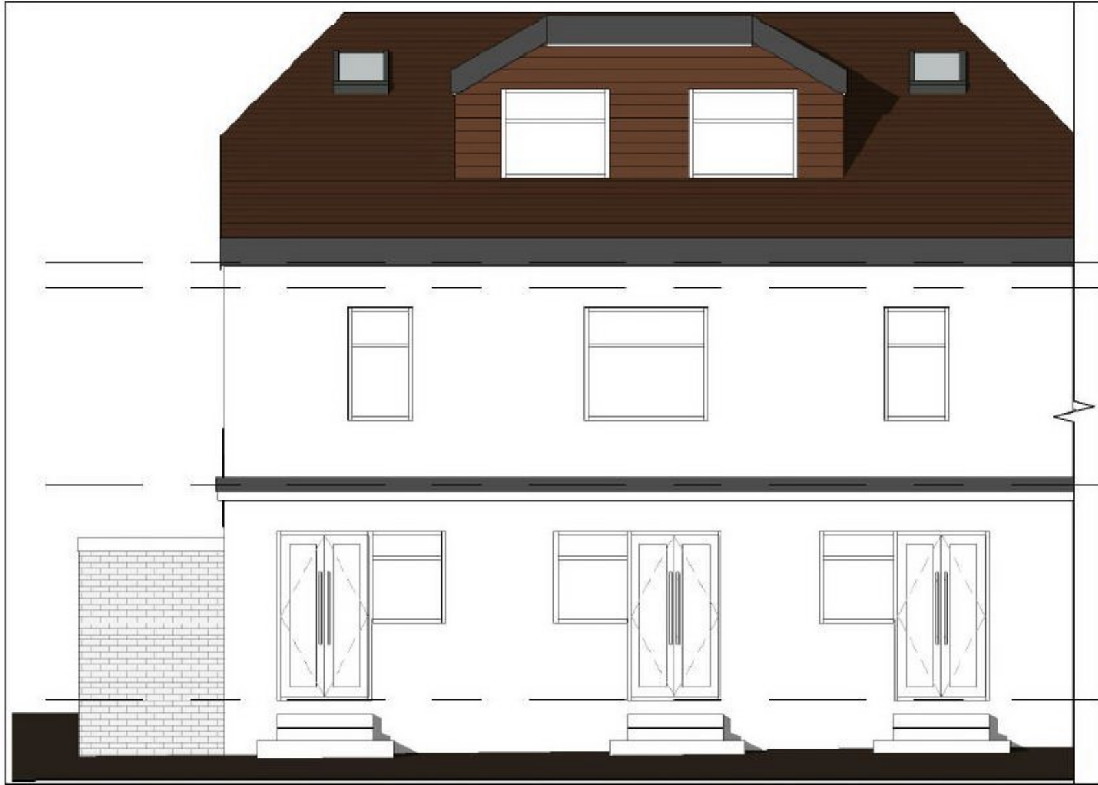
Proposed rear elevation of no.48 with smaller central rear roof dormer in the middle of the roof slope.
