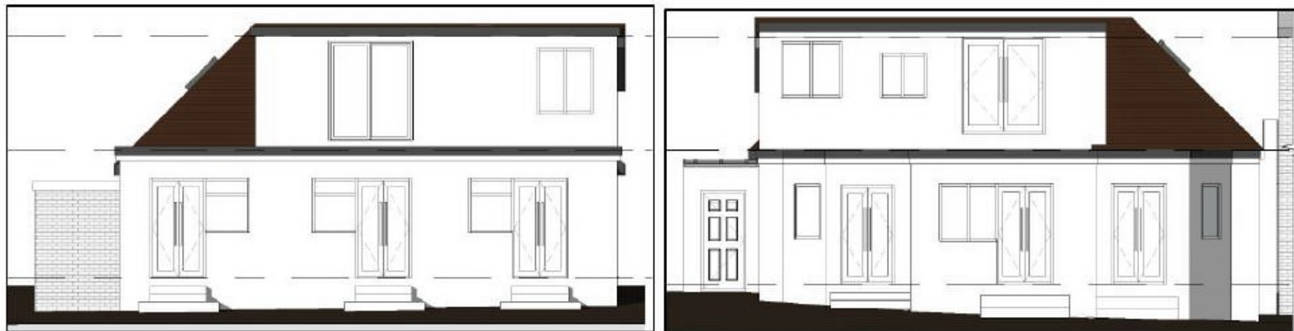
Existing rear elevations showing existing dominant PD roof dormers across the majority of the roof slopes.
