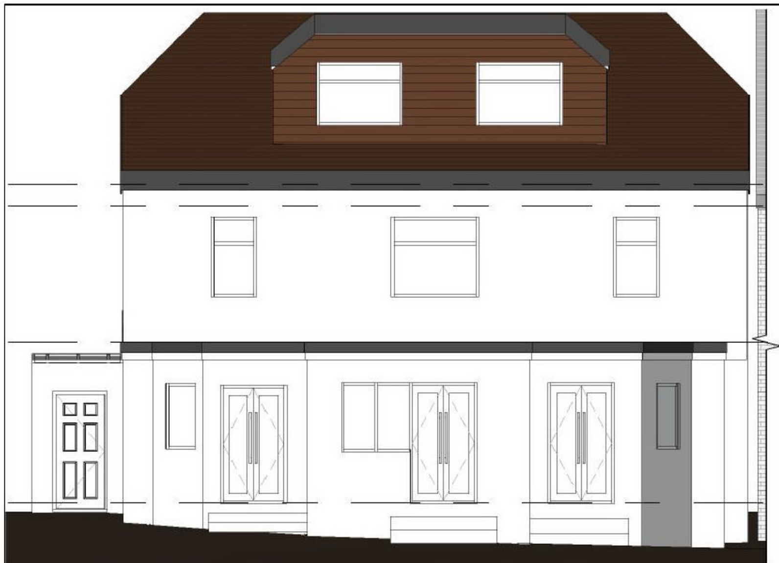
Proposed rear elevation of no.50 with smaller central rear roof dormer in the middle of the roof slope.
