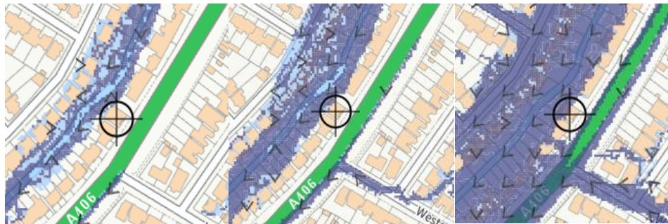
Figure 5a – High, Medium and Low risk scenario; surface water flood risk depth.
