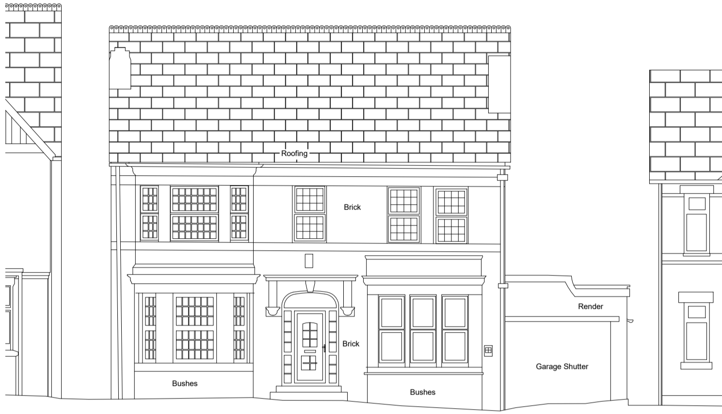
Front Elevation - Existing 1 : 100
