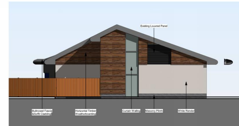
⑤ Existing West Facing Elevation 1 : 100
