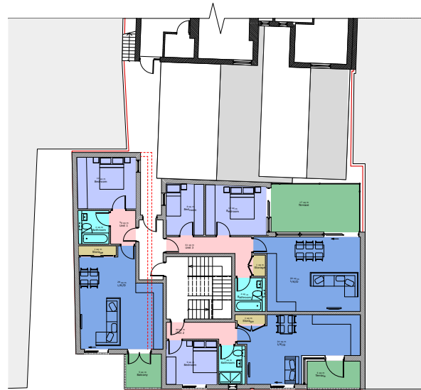
Fig 5. Proposed First Floor with wall demolition shown.
