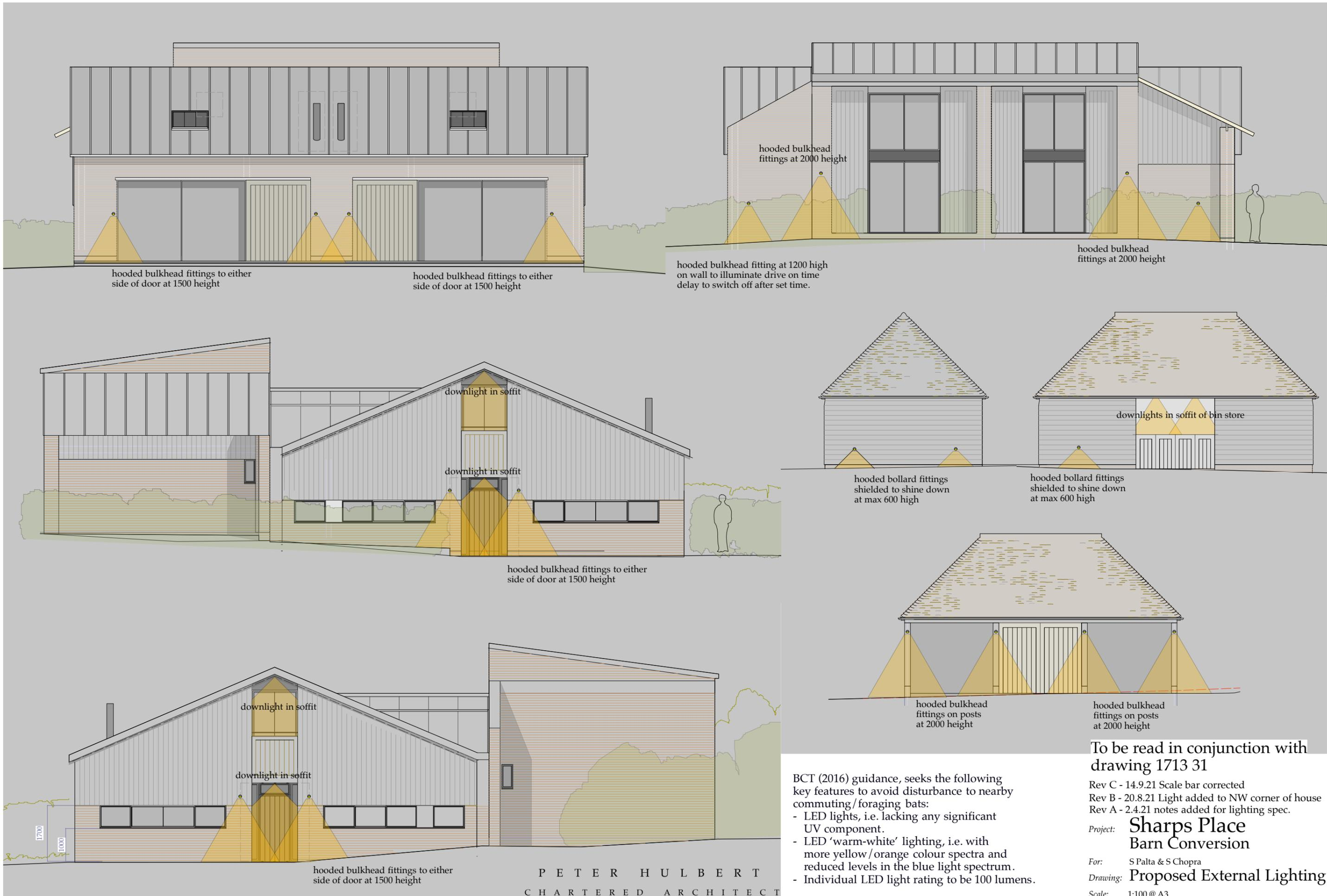
hooded bulkhead fittings to either side of door at 1500 height
