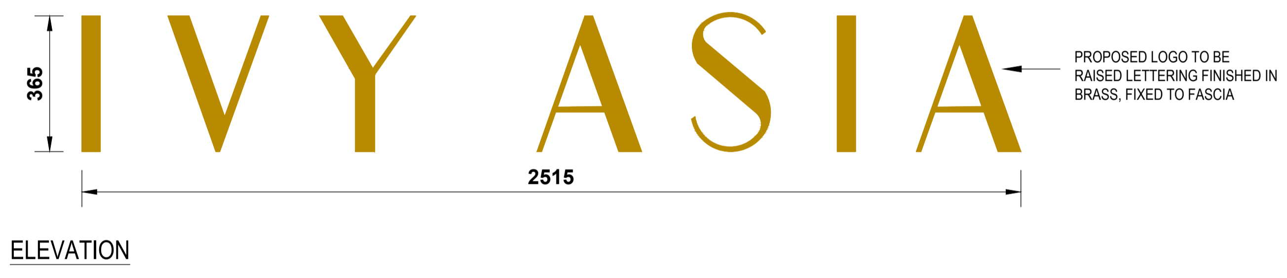
PROPOSED FASCIA SIGNAGE DETAIL SCALE 1:10
