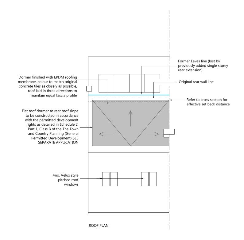
Drawing PD - 7 - Roof Plan (Proposed)
