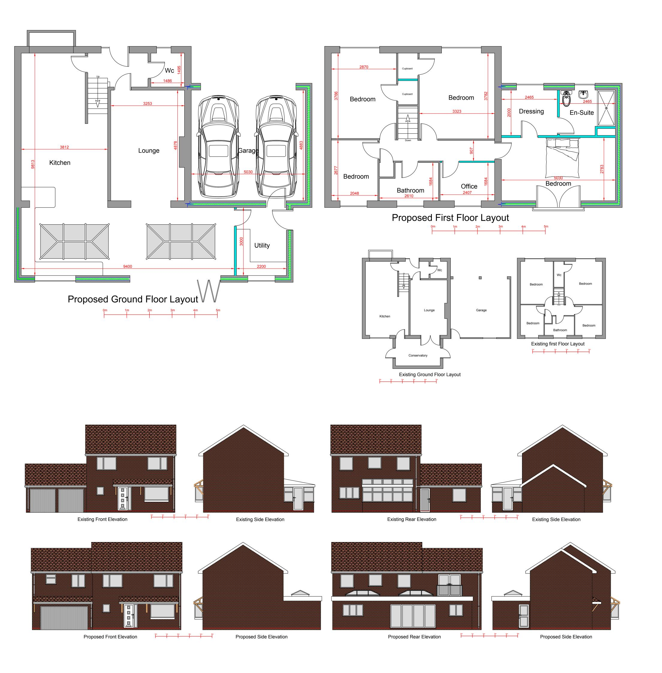
delete as necessary form Extension as shown 1: Windows to be double glazed with pilkington K,E glass with min 16mm airgap between glazing. Trickle vents fitted giving min 8000mm2 openers min $\frac{1}{20}$ th opening lights. Windows to be quality C or better 2: window and door openings to have draught seals fitted. 3:All glazing to windows within 800mm of floor & 1.5m in doors & side panels to be fitted with safety glass
