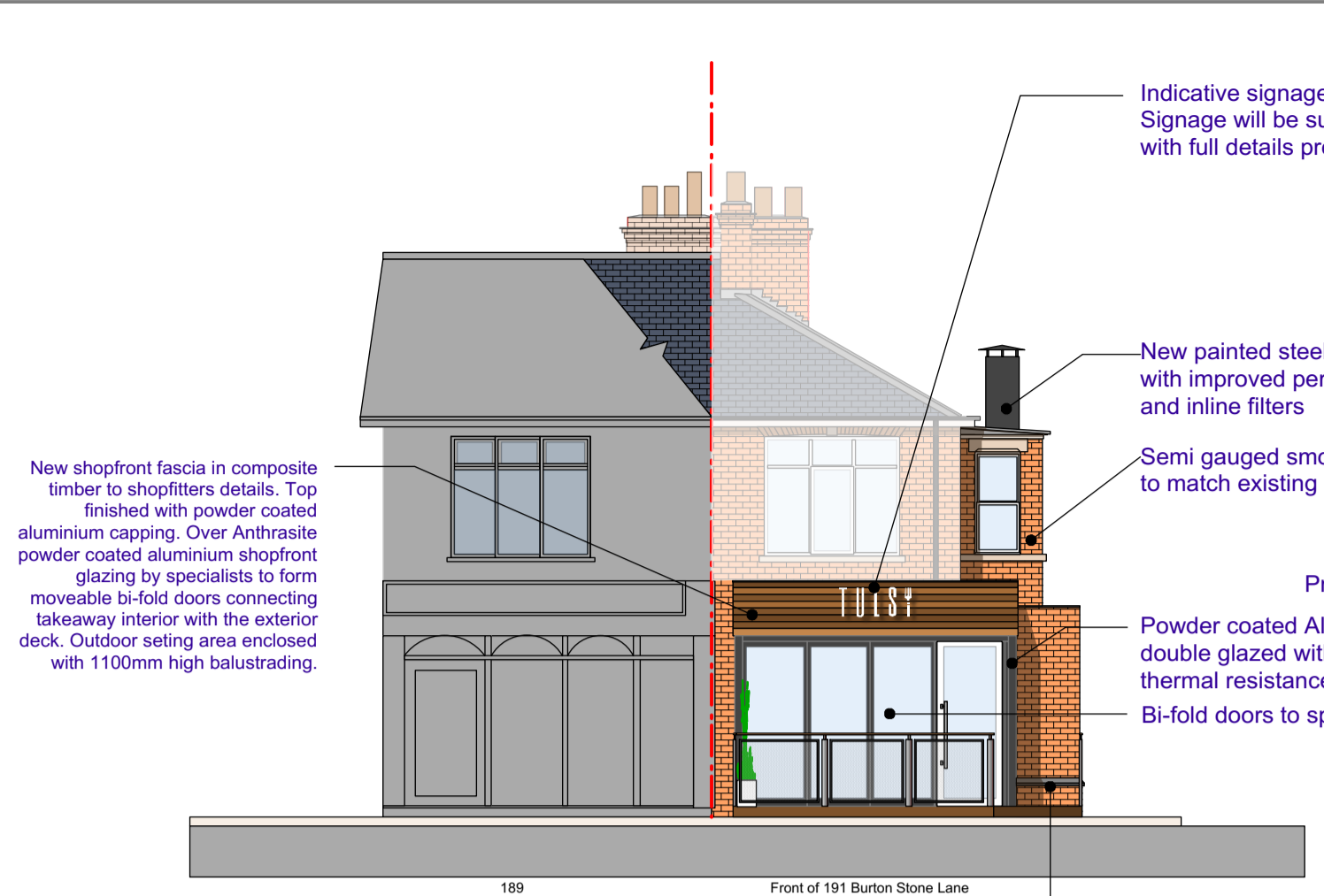
EAST ELEVATION - PROPOSED 1:100 Along Burton Stone Lane
