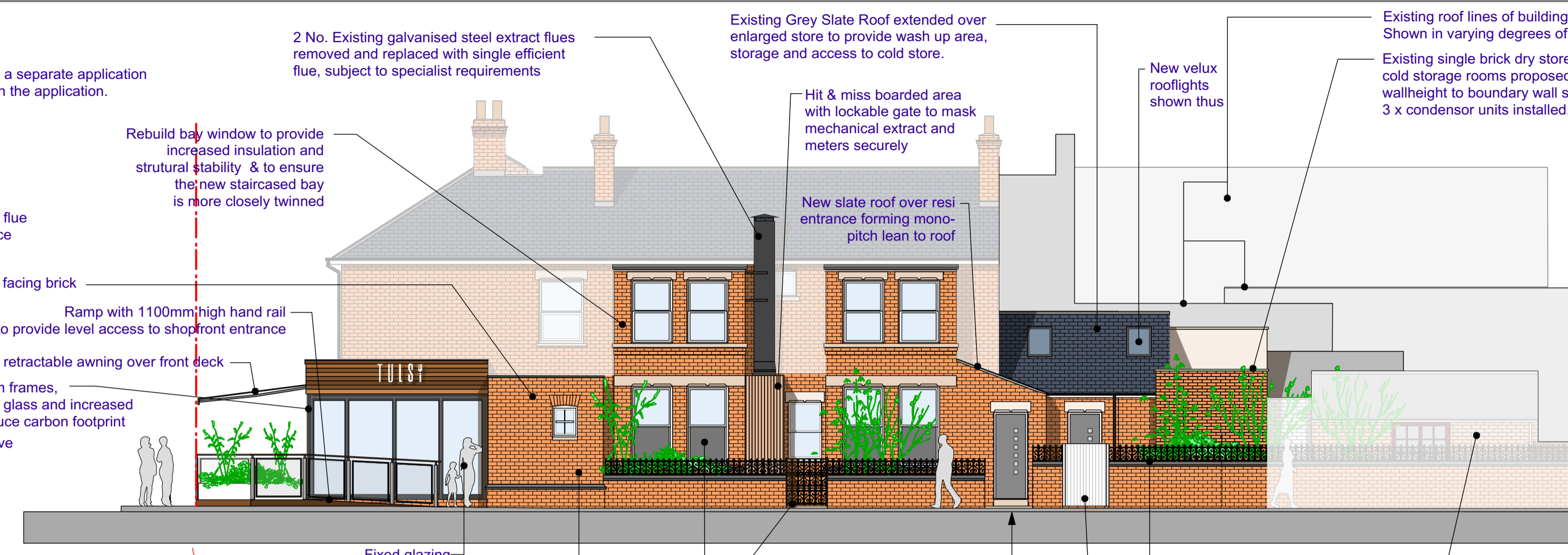
NORTH ELEVATION - PROPOSED 1:100 Along Garth Terrace
