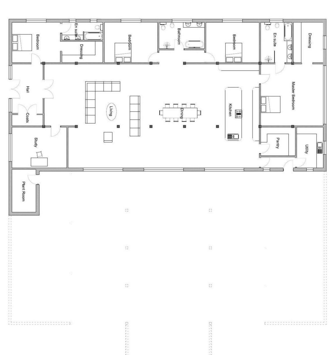
Proposed Floor Plan (Gross floor area 412 sq m)
