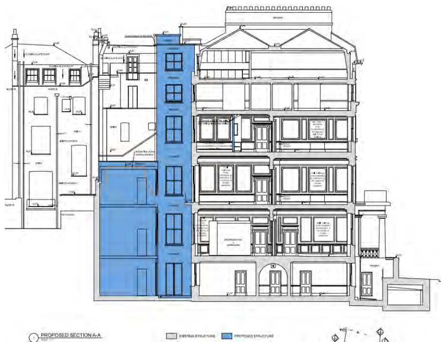
Figure 34: Section from 2018 application 18/05305/FULL for the division of the building into 3 residential flats indicating new windows over-looking number 3 and increased height which will increase sense of enclosure and block light.
