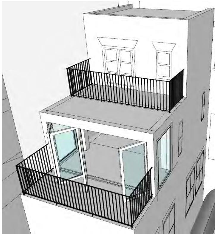
Figure 31: Proposals shown to give a further understanding of the overall form of the extension. The top balcony is set-back in order to reduce over-looking to adjacent properties.
