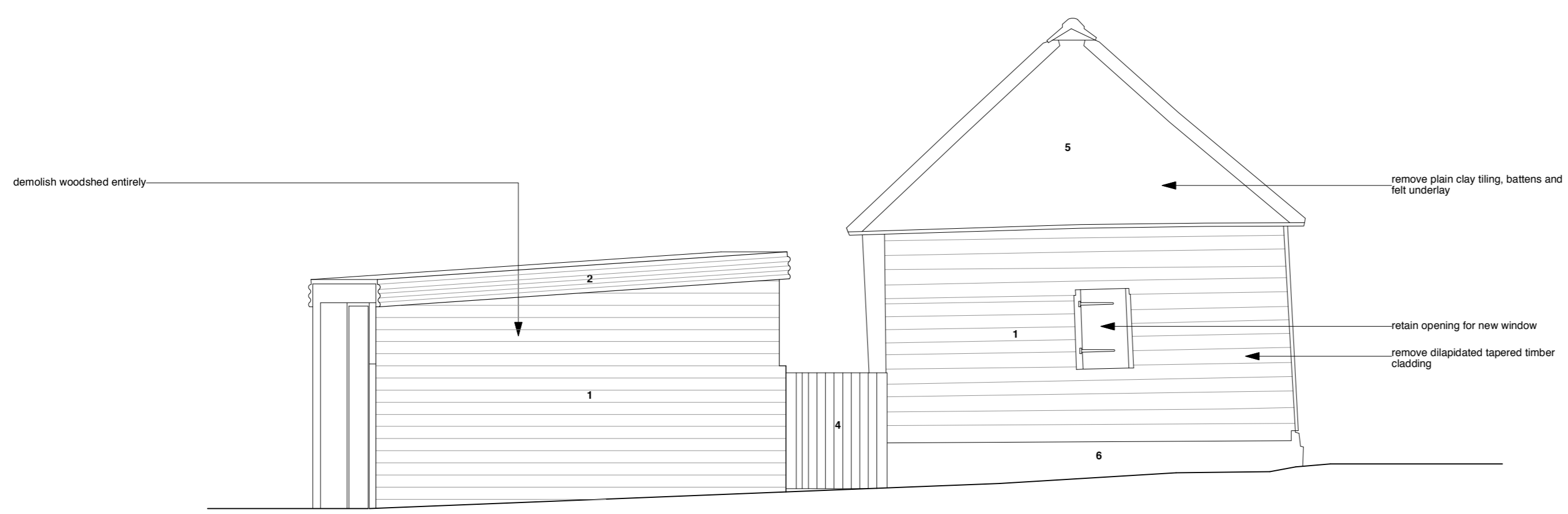
BARN and WOODSHED EAST ELEVATION AS EXISTING timber frame to existing barn to be retained
