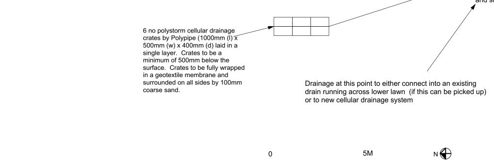
All dimensions should be checked on site. Do not scale from this drawing
