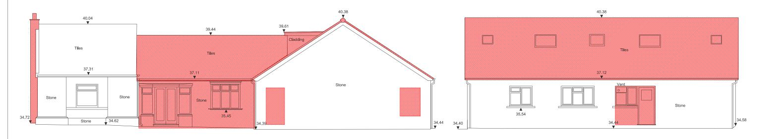
③ EXISTING EAST ELEVATION AREA TO BE DEMOLISHED HATCHED IN RED
