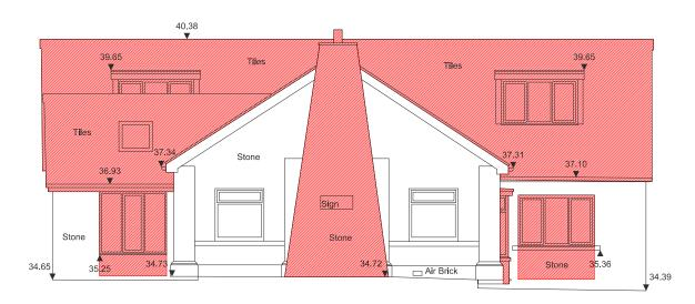
① EXISTING WEST ELEVATION AREA TO BE DEMOLISHED HATCHED IN RED
