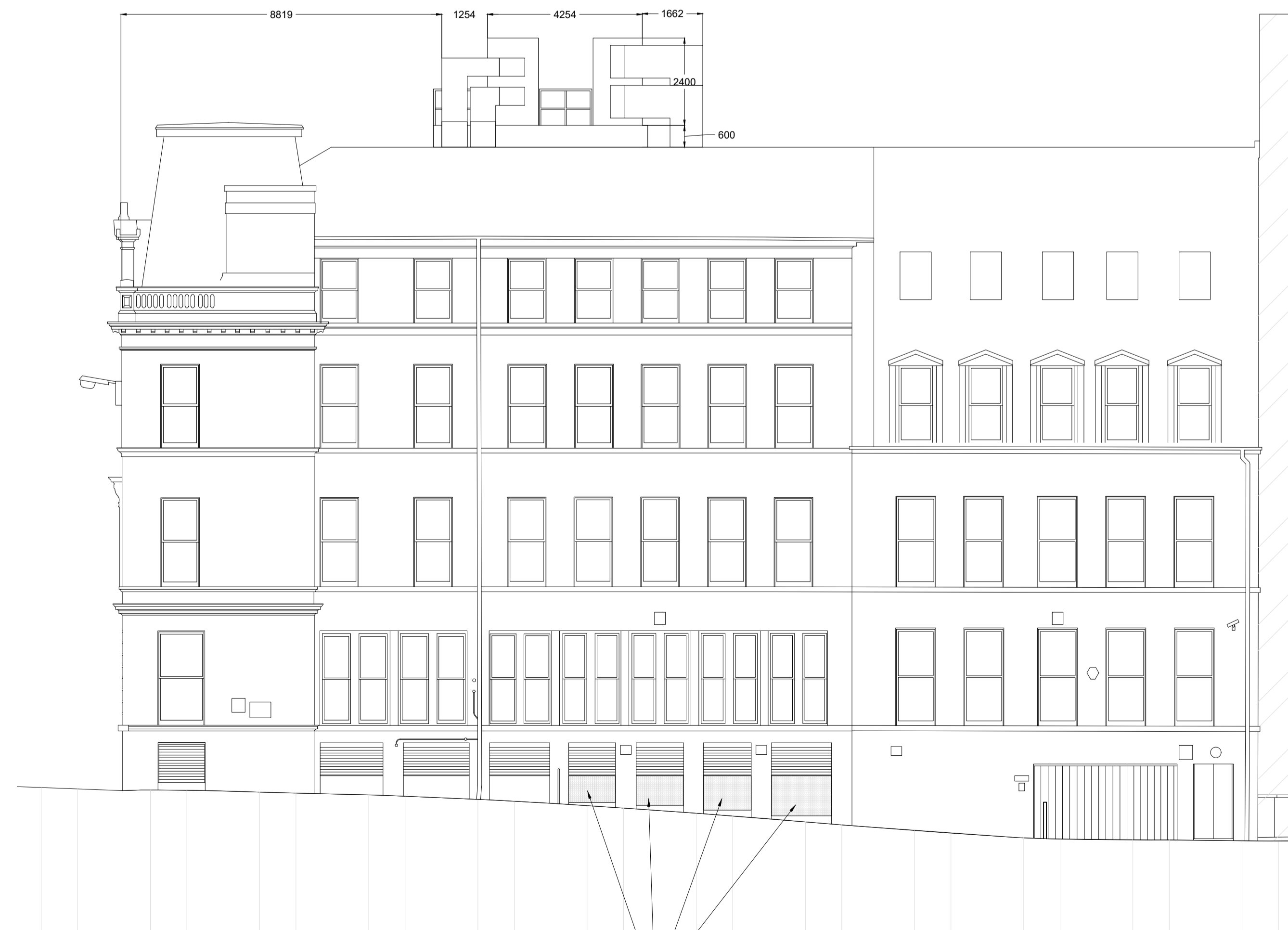
2 Bath Lane - Proposed Elevation 1:100 0m 2m 4m 6m 8m
