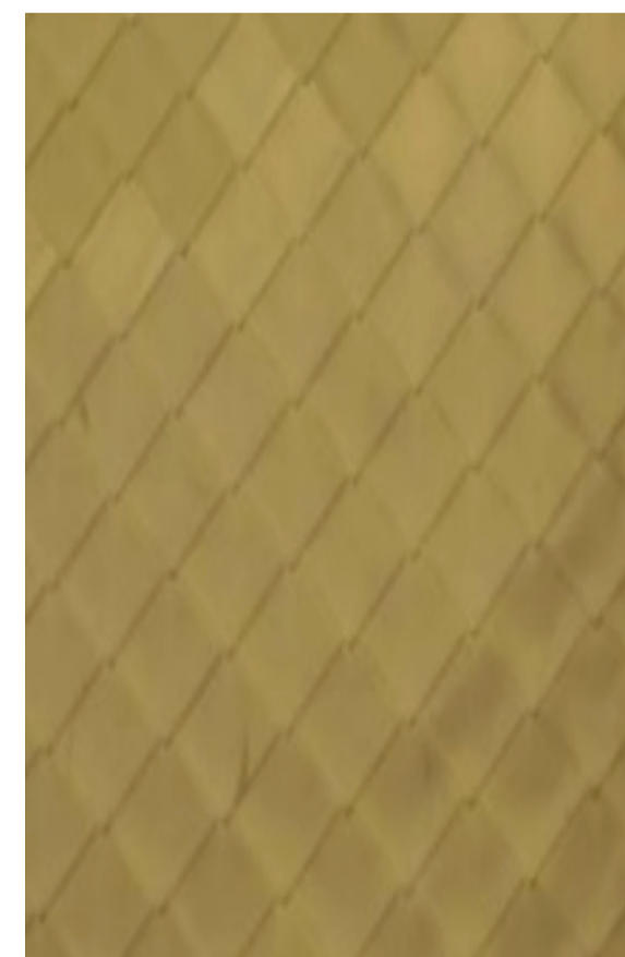
Tecu Gold metal shingles - 430 x 600 (weathers to a earth brown dark colour to blend with thatch)
