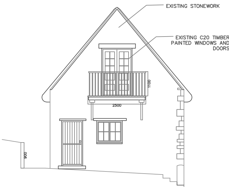
EXISTING SOUTH ELEVATION
