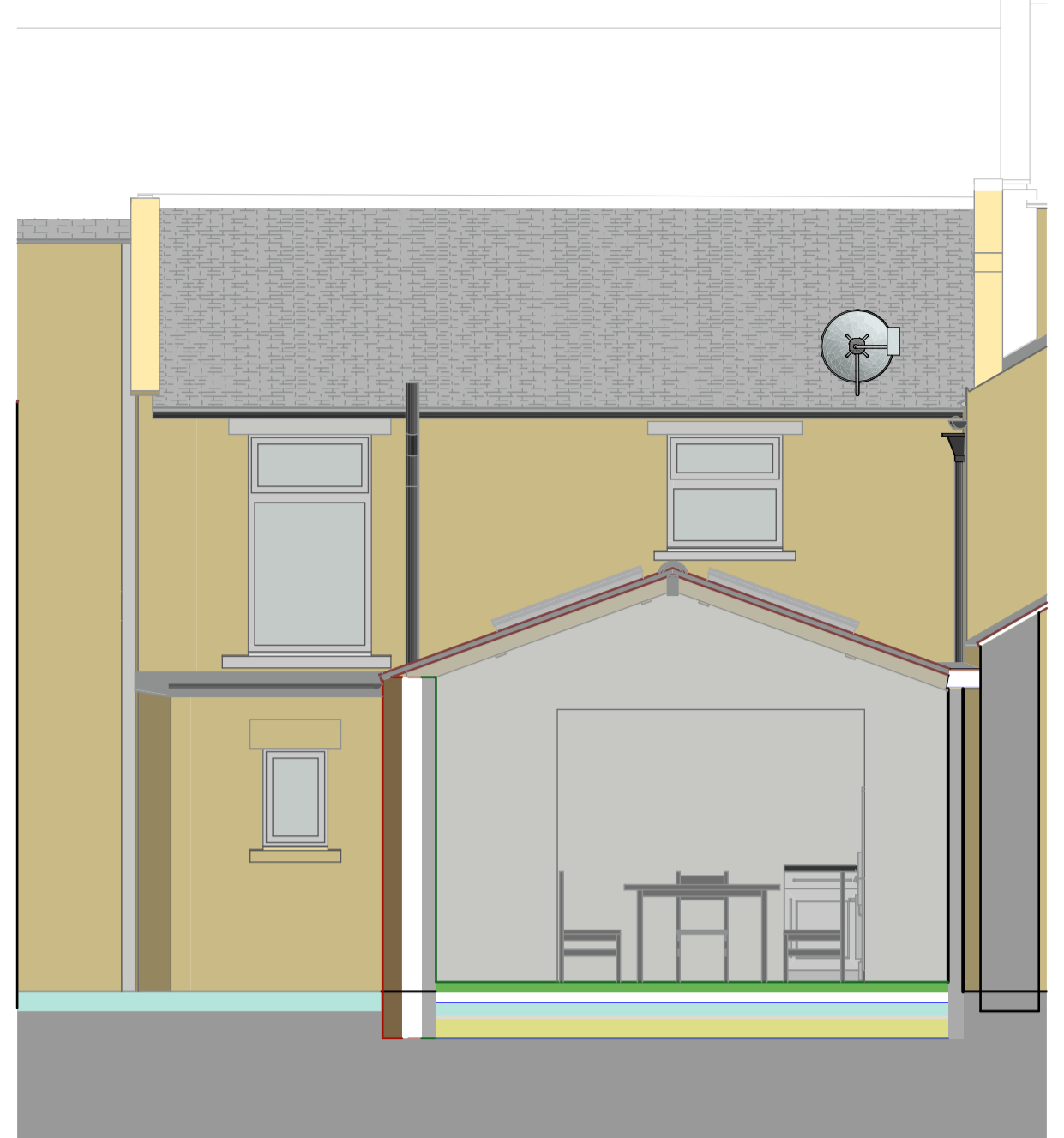
3 S-01 CROSS SECTION TO EXTENSION 1:50
