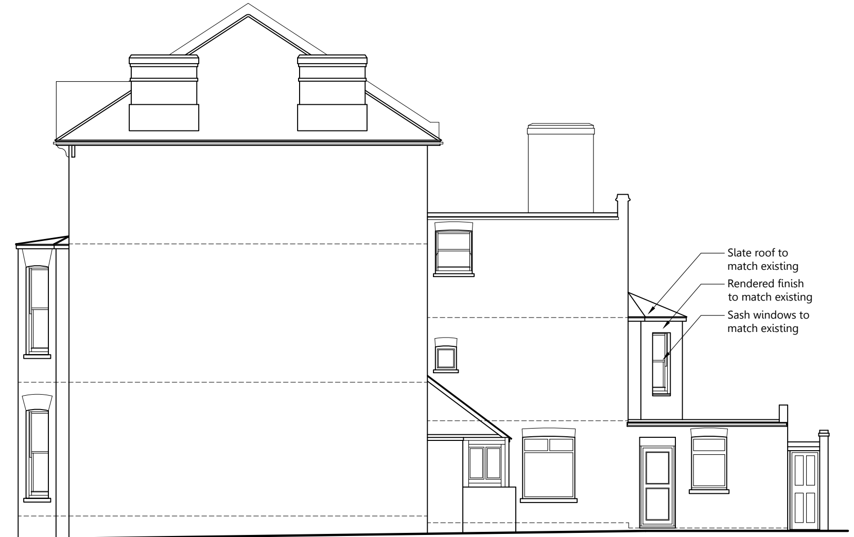
Side Elevation (south facing) Scale 1:100 @ A3
