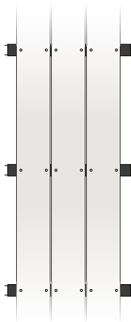
Fixed twice using Cedral colour matched screws or stainless steel ribbed coil nails
